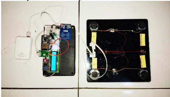
Gambar. 6 Wiring diagram timbangan IoT
